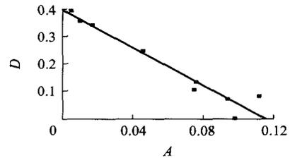
Fig. 8 Relation between amplitude and damage parameter
