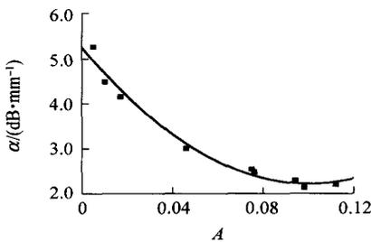
Fig. 6 Relation of amplitude and attenuation coefficient
