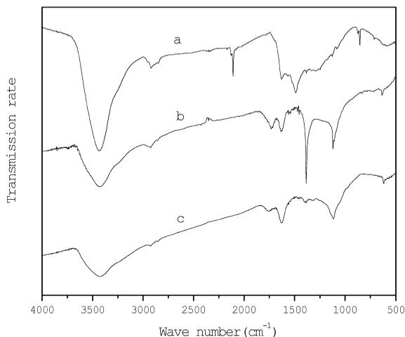
Fig. 4. FTIR spectra of the soot of TNT/RDX (50/50) in a water environment (curve a), the UFD purified by perchloric acid (curve b), and the UFD purified by a mixture of sulphuric acid and  $\text{KMnO}_4$  (curve c).
